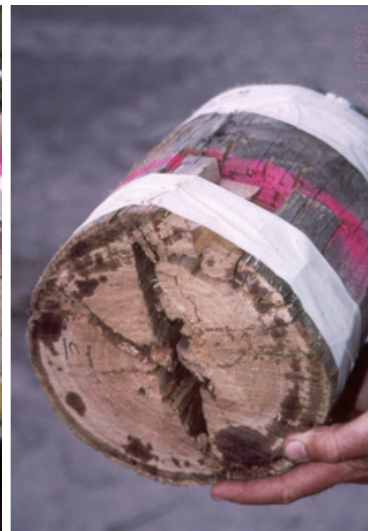
Pole sectioned to reveal extent of good wood
