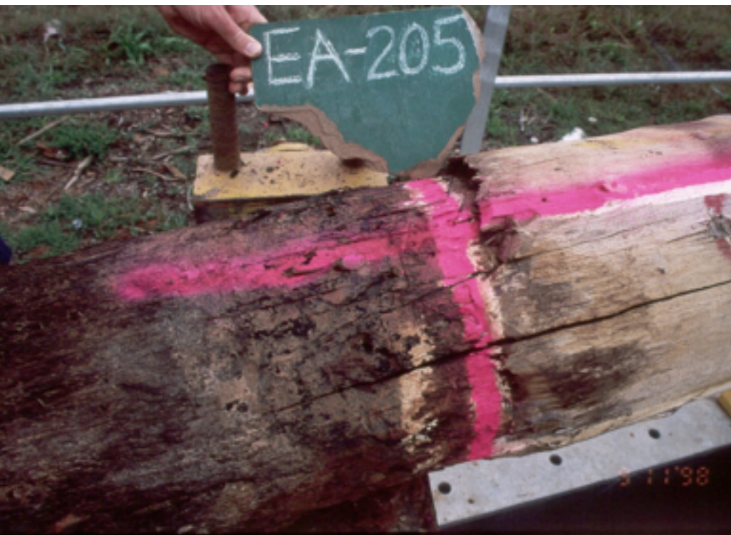
Condemned pole ready for further inspection
