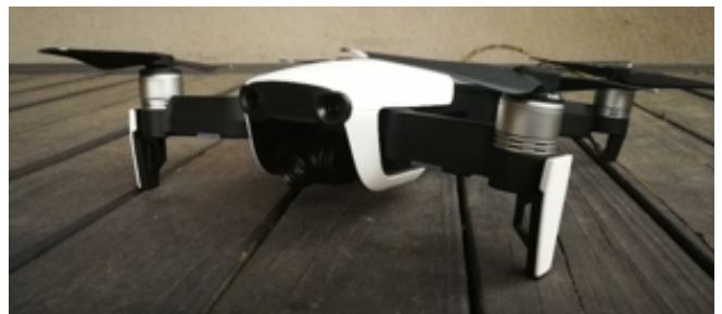
Figure 1 – Rotary wing RPA – DJI Mavic Air used to capture images in this paper
